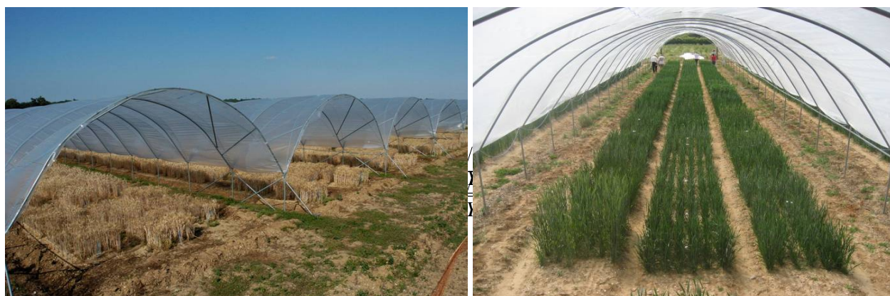
Figure 1. Polytunnels used to impose drought in 2007. The polytunnel system, which has only a minor effect on crop microclimate, is also used to screen for drought tolerance and water use efficiency in sugar beet (Ober ES, 2004).
