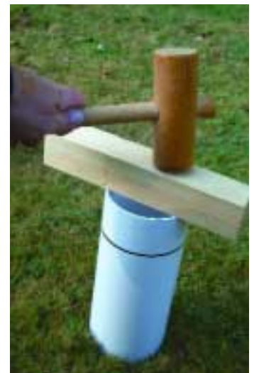
A plastic pipe driven in the ground is filled with brine.
