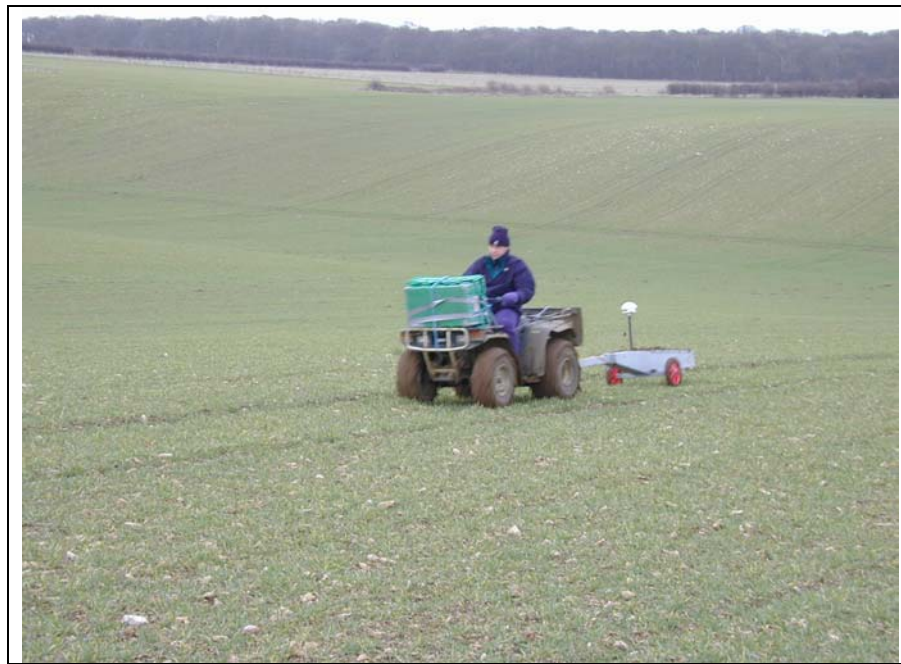
Figure 1. EMI equipment in cart drawn by an ATV.
